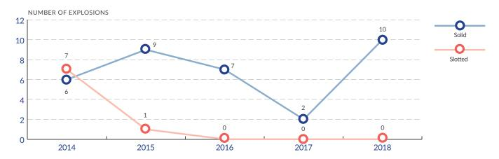
Slotted manhole covers are designed to minimize the impact of manhole events by allowing gas and smoke to vent from manholes in the event of an underground failure. Slotted manhole covers allow energy to disperse more easily when an event occurs, thereby preventing buildup of gases to potentially explosive proportions. The trade off when installing slotted covers is that they allow more water and street run-off contaminants to enter the manhole than solid covers.
