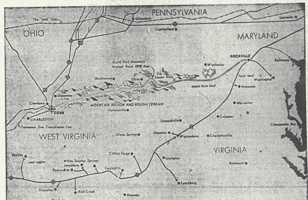
The route of the "Toughest Inch," the broad line between finer black lines are earlier installations and the broken lines are those of other companies. The crossed circles are compressor or booster stations
